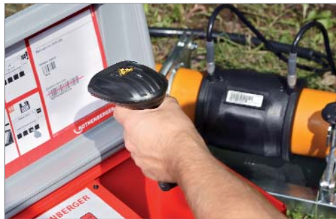
Name of the welder and the construction site can be scanned in easily
